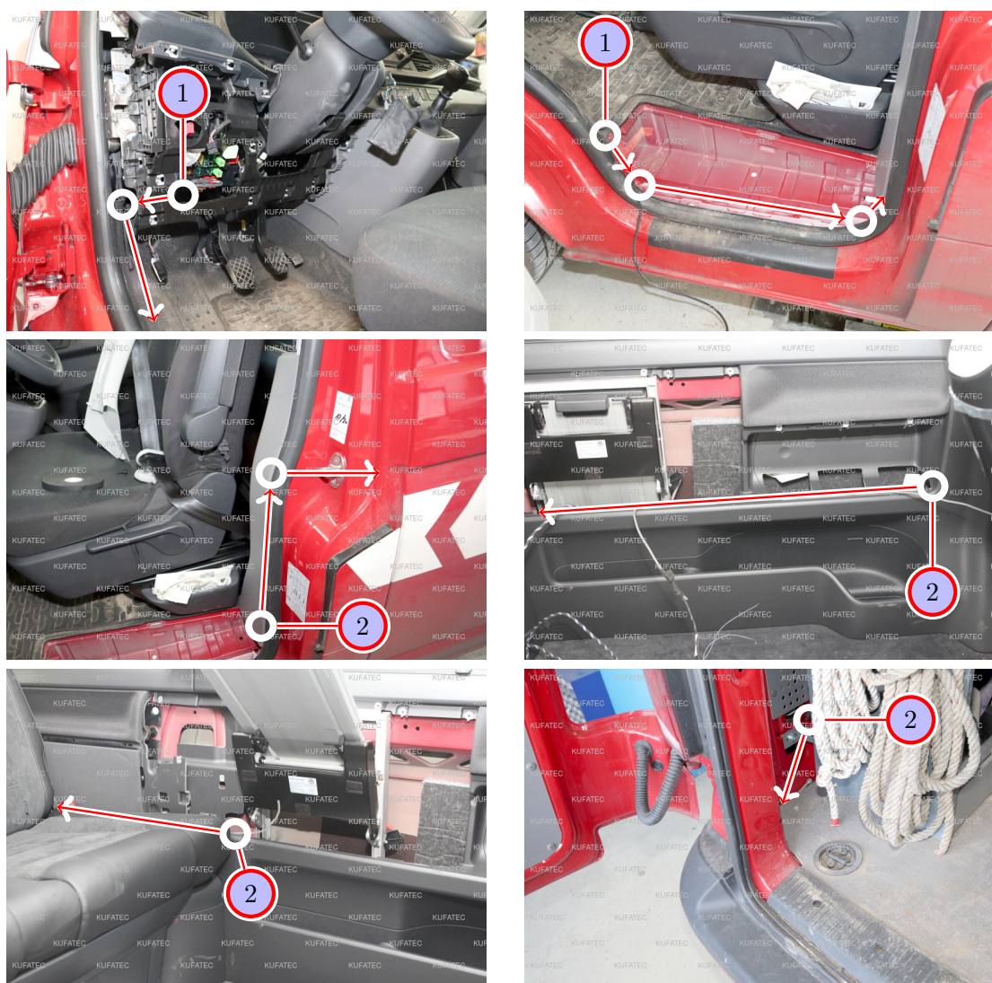
Figure 7: Cable routing driver's footwell to the back
